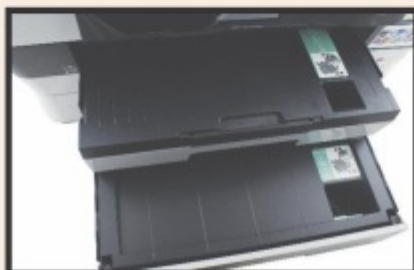
The Brother MFC-J3720 has two paper feeders that are capable of holding 500 sheets of paper in total
